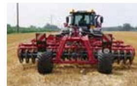
Easy conversion from working to transport position. The two-part hydraulic folding gives a transport width of max. 2.75m. The hydraulic suspension ensures smooth running and safe road transport.
