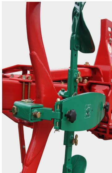
The Kverneland 2500 i-Plough® features legs with a new design, called "aero-profile". Not only higher than the standard Kverneland legs, these new legs improve the soil flow. Heavy residues are pushed out, hence limiting possible blockages regardless of the 85/100 cm interbody clearance.
