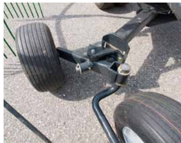
Tandem axle for two rotors
