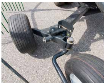
Tandem axle for two rotors
