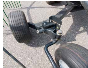
Tandem axle for two rotors
