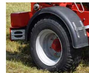
Mud guards reduce mud and dirt building up on the pre-stretcher and film rolls when operating in soft ground field and during transport.
