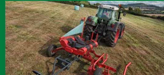
Turntable with two driven rollers designed for a high bale stability and smooth even rotation.
