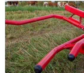
The adjustable loading arm allows the bale to be picked up and loaded on the move.
