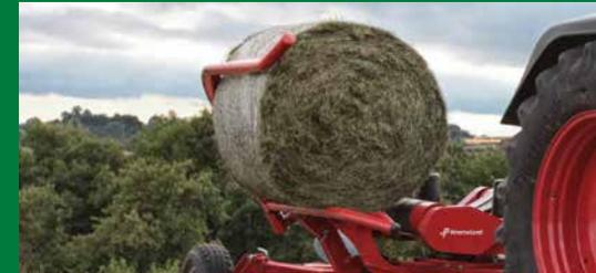
Hydraulically operated loading arm, and a low loading height, provides fast transfer of bale from arm to turntable.
