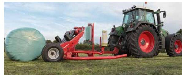
Low design of the machine ensures fast and gentle unloading of the bale.
