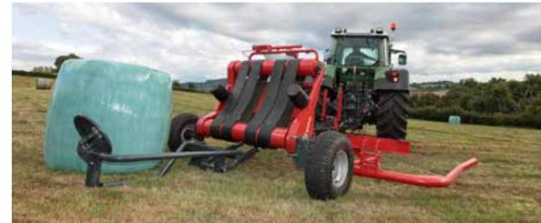
The Kverneland Turntable wrappers can be fitted with a bale on end kit.
