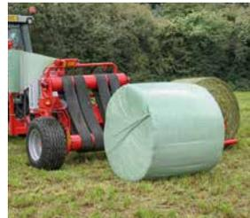
Fast and gentle on-the-move unloading with no need for a fall damper.
