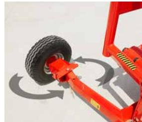
To achieve a narrower transport width, the right hand wheel is turned to the inside of the support arm.
