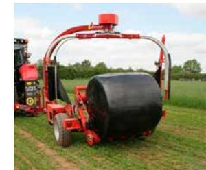
Fast and gentle unloading of bales with no need for a drop mat.
