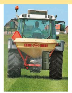
Border spreading with the border spreading plate
