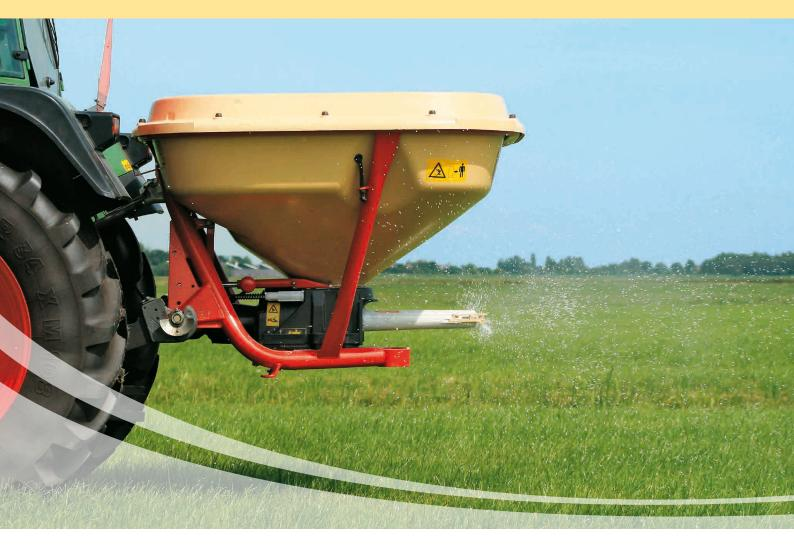
More than one million machines sold prove that the Vicon pendulum seeder/spreader is the first choice wherever the demand is for maximum accuracy in fertiliser application. Spreading quality and ease of operation of this unique machine are unequalled - now as in the past. The pendulum movement of the spout ensures that the application rate is always identical on both sides. This results in an excellent overlap.
