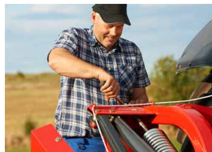
Easily adjustable suspension springs.
