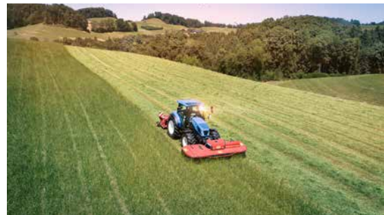
EXTRA 332XF Compact with gravity point close to the tractor is an important feature when operating in hilly conditions with smaller tractors.
