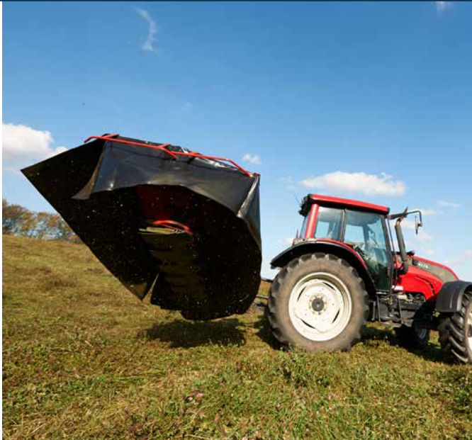
Lifting on headlands via a hydraulic cylinder.
