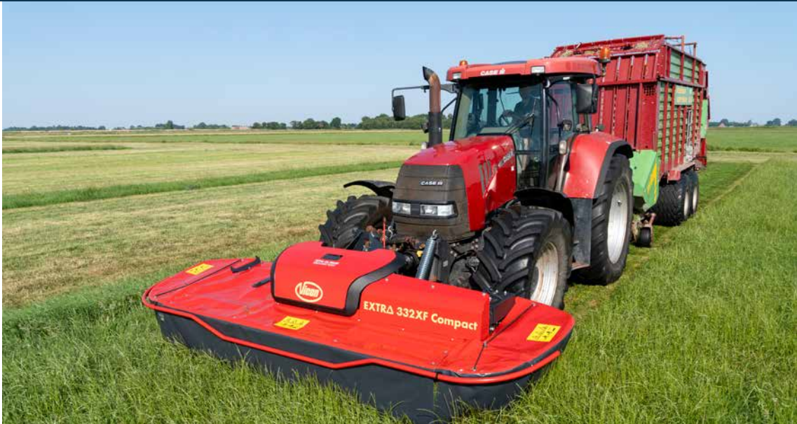
Zero grazing application with a loader wagon, running at low forward speed.
