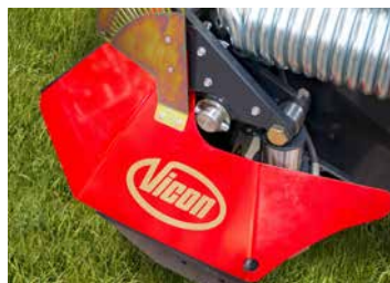
Hydraulic on-the-go setting of ground pressure (optional).
