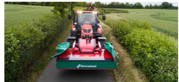
Hydraulic folding of FlexProtect guards (optional).
