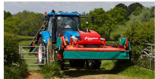
Foldable sideguards ensure narrow transport width.
