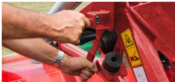
One-touch parking handle, to lock and prepare the machine for dismounting.
