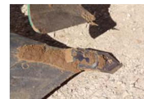
Soil flow protects other parts.
