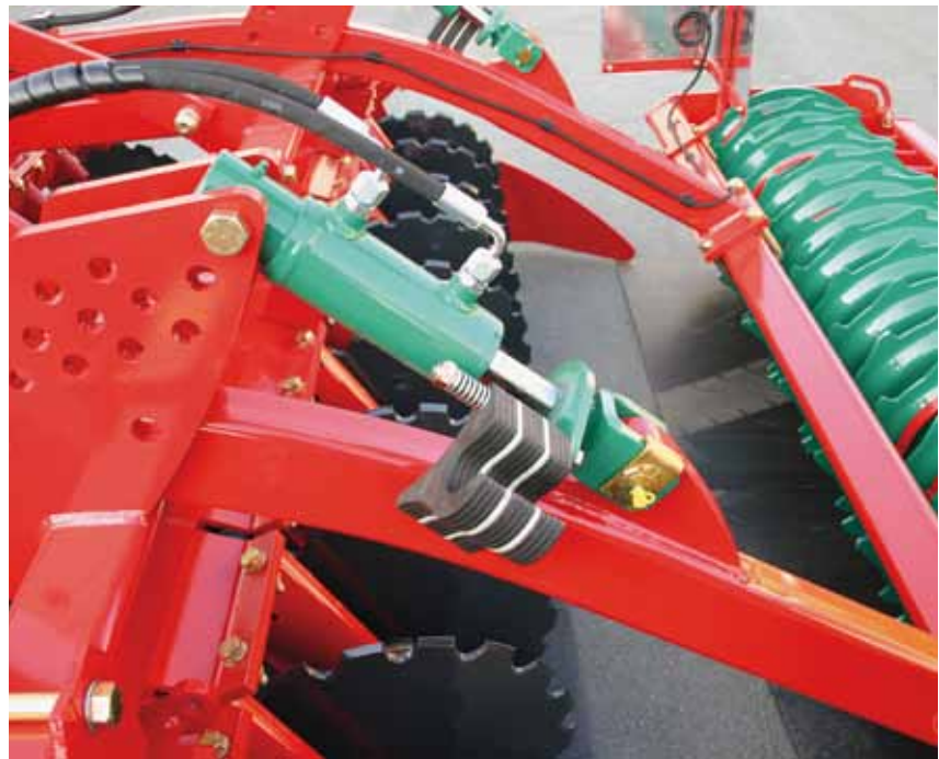
Figure 2: Hydraulic adjustment of the working depth
