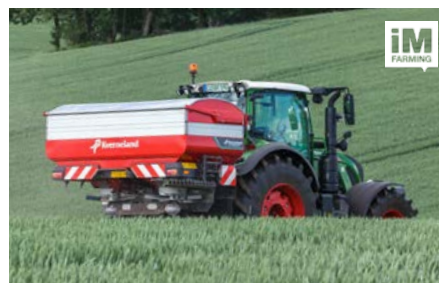
Exacta-CL/TL/TLX GEOSPREAD® Unnecessary overlap is set to a minimum, because of section control. The total benefit of GEOSPREAD® combined with speed related spreading and GEOPPOINT® headland management can be up to 15%. The GEOSPREAD system does section control with sections of only 1 metre.
