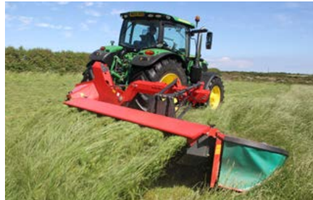
3300 MT/MR Series QuattroLink mowers with dual adjustment of conditioner plate. Available with 400 mm hydraulic on-the-go Vario adjustment.
