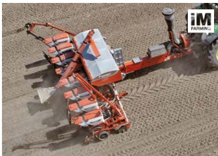
Optima TFprofi (trailed) Reduced tractor power requirement and large hopper capacity for maximum operating efficiency. The Optima TFprofi is available with HD-II and SX sowing units. An optional central seed hopper of 870 L together with SX rows increases the performance and reduces the set-up time.
