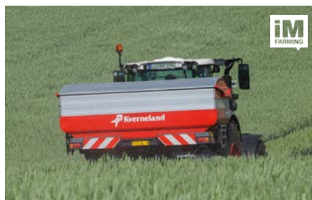
Exacta-TL The weighing system with automatic calibration helps to prevent over and under dosing which will result in better yield.
