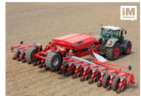
Optima TFmaxi (trailed) For high performance with 16 HD-II rows and a 4,000 L capacity fertiliser hopper.
