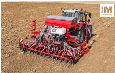
Pneumatic Mounted Seed Drill e-drill maxi plus Seeding and fertilising in one pass. The hopper capacity of max. 2,100 litres is divided into an adjustable ratio of 60:40, 70:30 or 100:0. With two independently working ELDOS either side.
