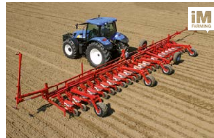
Monopill rigid (3 m, 6 m, 9 m & 12 m) Designed for high output and quick exchange between road and field. From 6.0 m, available with lengthwise transport device.
