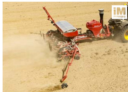
Optima TFprofi (trailed) Reduced tractor power requirement and large hopper capacity for maximum operating efficiency. The Optima TFprofi is available with HD-II and SX sowing units. An optional central seed hopper of 870 L together with SX rows increases the performance and reduces the set-up time.
