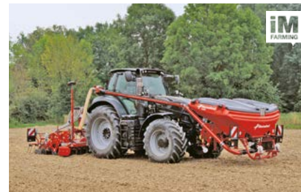
Front hopper f-drill & coulters bar f-drill CB F The ISOBUS controlled front hoppers f-drill compact (1600 L) or f-drill maxi (2200 L) with one ELDOS metering device or two as duo or plus version ensuring high application rates. The f-drill maxi plus enables to applicate two products in one pass. It is the real partner to combine with strip tillage, cultivator, short disc harrow, weeder, power harrow coulters bar or precision drill. In combination it offers even weight balance and maximum flexibility.
