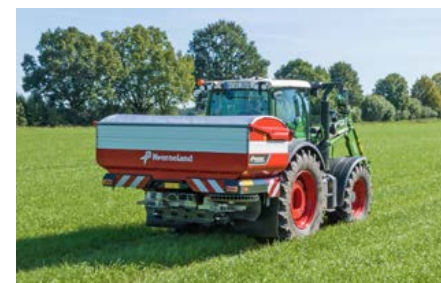
Exacta-TL/TLX GEOSPREAD® iDC iDC means intelligent Disc Control. Due to the possibility of the independent disc speed left and right this can be used during border spreading. To have a perfect spreading pattern at the border of the field the disc RPM can be decreased on the border side.
