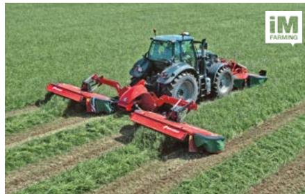
5387 MT BX Machine with 8.7m working width, QuattroLink suspension and dual adjustment of conditioner plate. Optionally available with BX belt.
