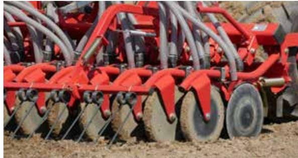
Thanks to the very slim design of the **CD coulters**, there is only a small amount of soil being moved. Therefore you need less pressure to achieve the right seeding depth. Thus, more of the available coulters pressure can be led to the press wheels. The result is a very even seed application.
