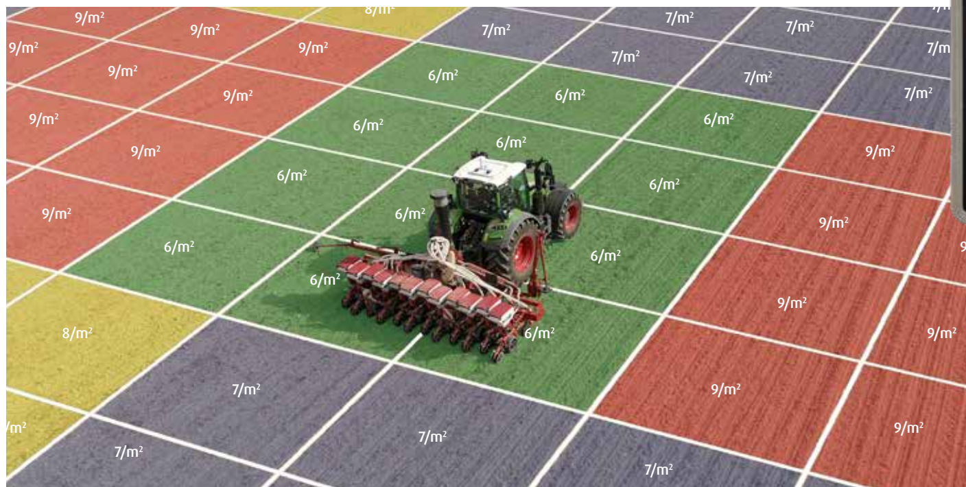
Example maize 60,000 to 90,000 seeds/ha depending on yield expectation and soil condition. Grid 5 x 5m.
