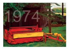
Kerteminde is the first manufacturer to combine a disc mower with a conditioner. With the Taarup TSC 2100, the mower conditioner concept is born. This is a new and more efficient system that both cuts and wilts the crop in one pass.
