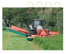
Kerteminde is among the very first to introduce an entirely new concept within mowing. With the triple-mower or butterfly concept, a massive 9 meter working width is achieved using a front- and two rear mounted mower conditioners.
