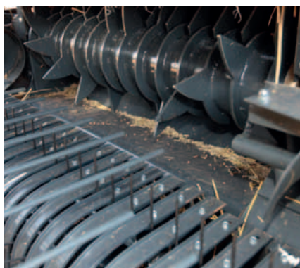
The PowerFeed rotor gives positive intake in all conditions.
