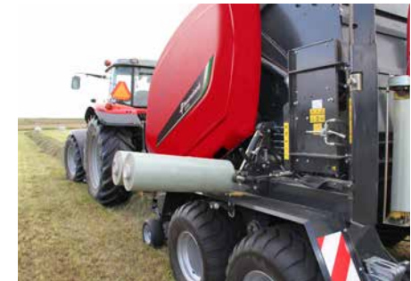
Twin cassettes for 10 spare film rolls operated hydraulically.
