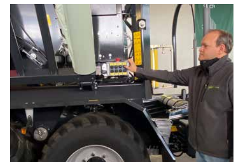
Twin cassettes for 10 spare film rolls operated hydraulically.
