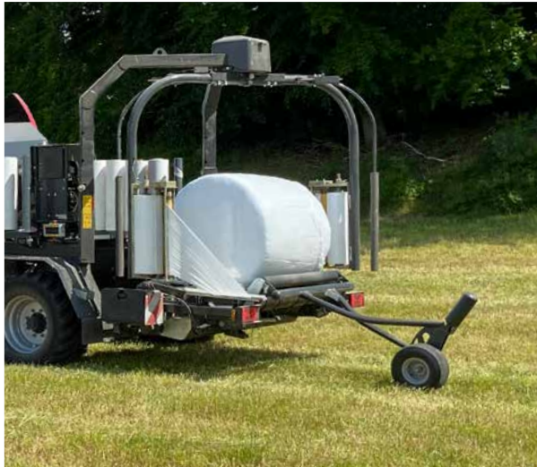
Twin satellite wrapper with 2 pre-stretchers and 4 endless belts for fast and stable wrapping.
