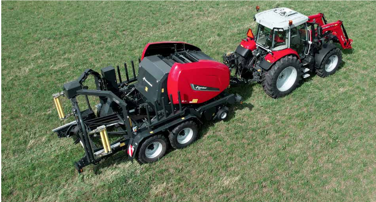
Twin satellite wrapper with 2 pre-stretchers and 4 endless belts for fast and stable wrapping.
