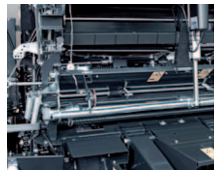
Twin tube fast operating twine binding system.
