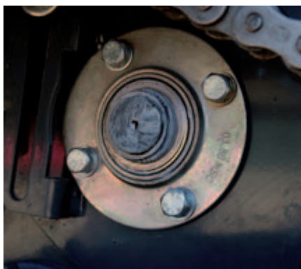
Each roller is carried on heavy duty bearings.
