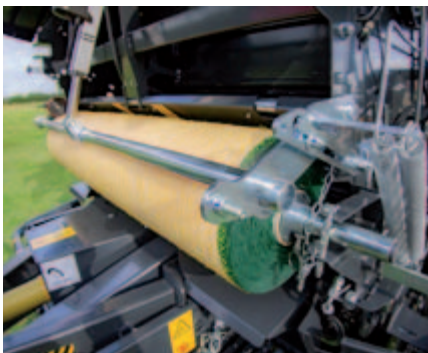
New high efficiency PowerBind net wrap system.
