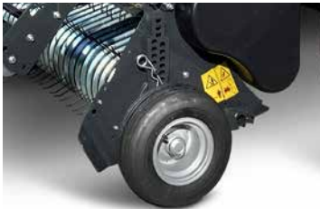
Large diameter easily adjustable guide wheels.
