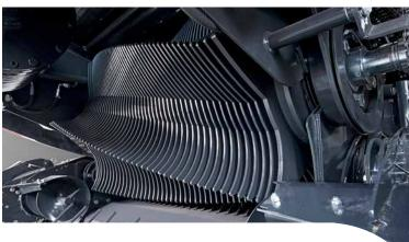
Equipped with 50 Hardox® tines, FastBale has unrivalled intake capacity. Close mounting of the pick-up to the rotor eliminates any dead areas when working in short crops.
