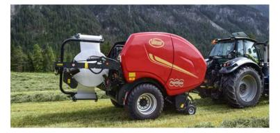
The innovative wrapping system breaks new ground for compactness. During transport, the rear roller and satellites are folded to the vertical position, considerably reducing overall length, while all wrapping elements are safely clear of any obstructions. Film rolls are also protected during transport by the satellite arms. The minimal tail swing allows easy access to even the tightest fields and gateways.
