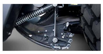
The 25-knife SuperCut chopping system features group selection giving a choice 6, 12, 13, 25 knives to match all conditions, all backed up with the security of a drop floor in case of blockage.
