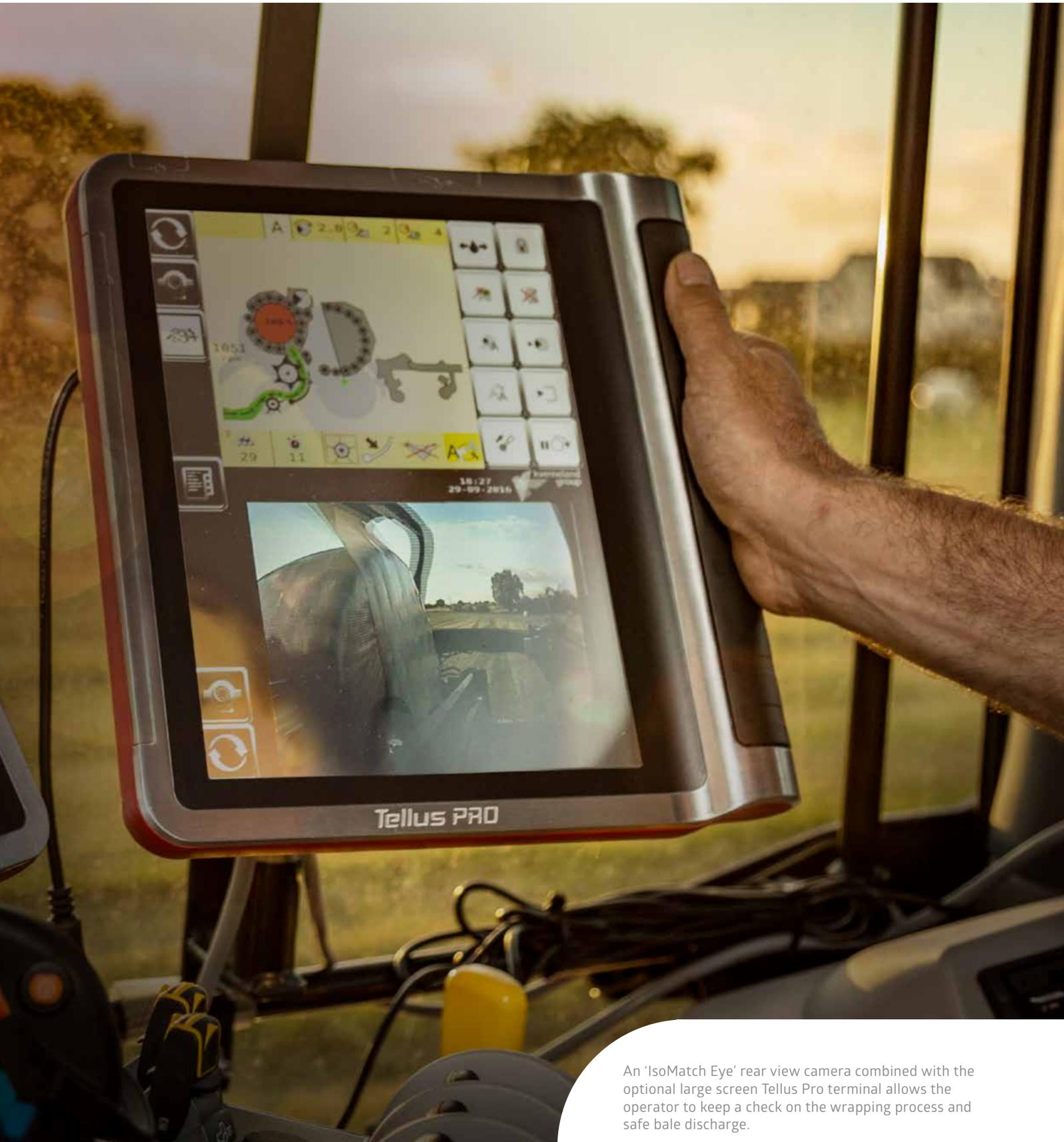
An 'IsoMatch Eye' rear view camera combined with the optional large screen Tellus Pro terminal allows the operator to keep a check on the wrapping process and safe bale discharge.
