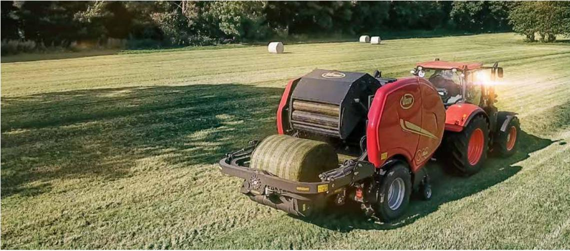
**“Completed bales are discharged directly onto the wrapper”**
