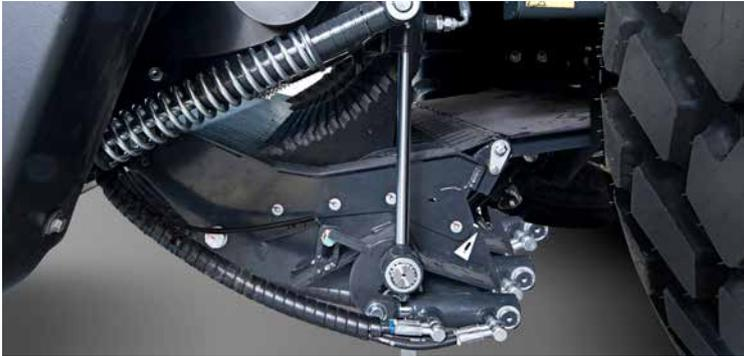
The 25-knife SuperCut chopping system features group selection giving a choice 6, 12, 13, 25 knives to match all conditions, all backed up with the security of a drop floor in case of blockage.
