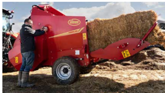
Operating both tailgate as well as floor chain in a safe distance from the moving parts by using the remote control placed on the side of the 860 series.
