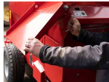
Adjustable slide for guiding material away from the wheel of the bale chopper.
