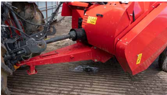
The extended drawbar ensures easier operation, especially when turning with larger tyred tractors.
