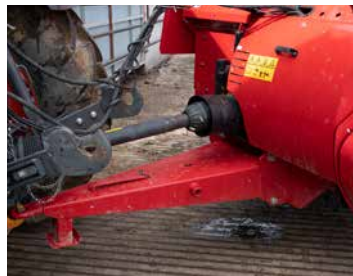
The extended drawbar ensures easier operation, especially when turning with larger tyred tractors.
