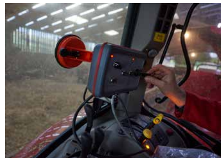
The 4-stage swivel chute is operated by the intuitive controlbox joystick.
