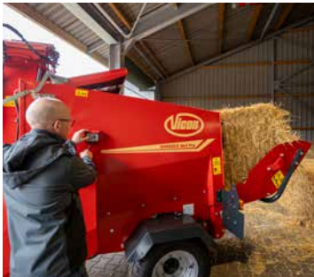
Operating both tailgate and floor chain in safe distance from the moving parts, by using the remote control placed on the side of chamber.
