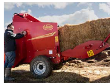
Operating both tailgate as well as floor chain in a safe distance from the moving parts by using the remote control placed on the side of the 860 series.
