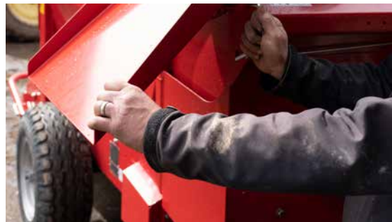
Adjustable slide for guiding material away from the wheel of the bale chopper.
