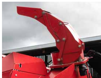
4-stage swivel chute for more accurate guidance of material. Especially when using the feeding application.
