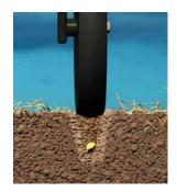
The Press Wheel firms the soil around the seed, optimising seed-to-soil contact, creating the ideal situation for germination, leading to consistent emergence.
