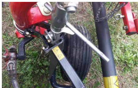
Optional third wheel lead to even more accurate track following and better tedding action.
