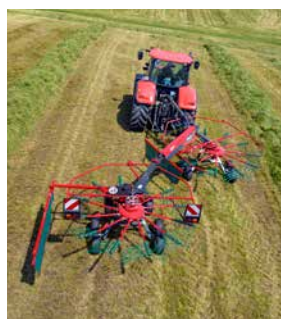
SideShift to the right - easy cleaning of borders with perfect view on the rotor.
