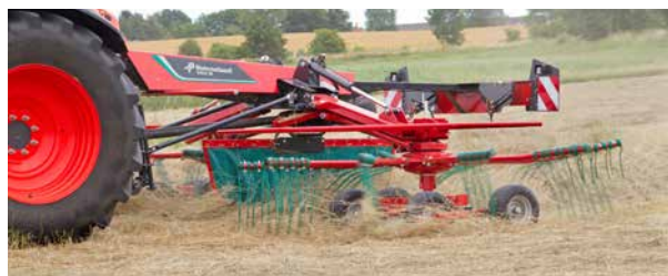
Better ground adaptation compared to larger single rotor rakes.
