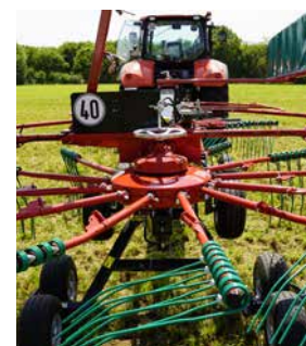
Easy adjustment of rotor height in the back.
