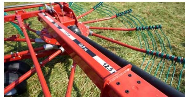
Hydraulic adjustment of working and swath width.
