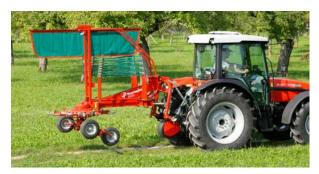
For transport or storage, the rotor guard frames are folded up close to the mainframe, locking automatically into position. An assistor spring linked to the swath board reduces the effort required.
