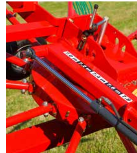
9476 C - Hydraulic 7.0-7.8m working width.
