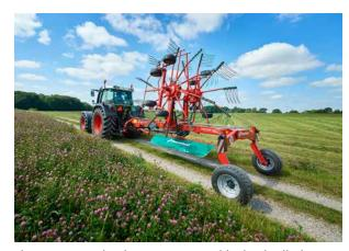
The centre swath rakes are converted hydraulically for transport from the tractor cab.
