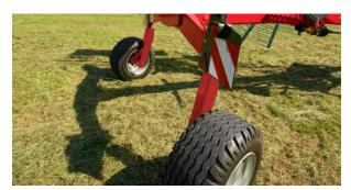
Active wheel steering for improved manoeuvrability in combination with large wheels for reduced compaction.
