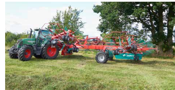
All four rotors can be lifted individually.
