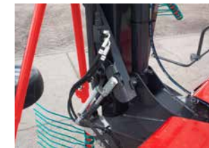
Hydraulic transport locking (optional).
