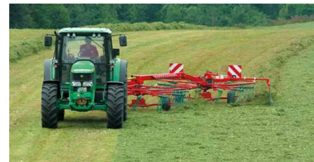
SideShift to the left - raking without driving on unranked crop.
