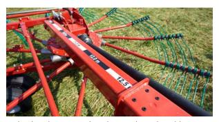
Hydraulic adjustment of working and swath width.
