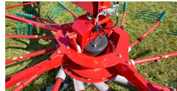
Each rotor can be independently and hydraulically set for height.
