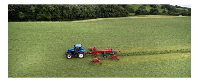
Correctly adjusting and customising the rake to the exact conditions you are facing today is what adds the extra quality to your forage, ensuring that dirt stays out of the swath, yet leaving no crop behind. Setting the rotor height, adjusting the swath width and fine tuning the cam track (ProLine) is done easily and intuitively on all Kverneland rakes, taking the hassle out of the daily work optimisation.
