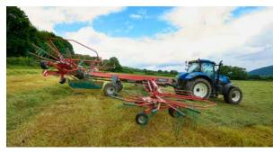
Individual pairwise lift of front and rear rotors. Adjustable time delay for headland position is standard.
