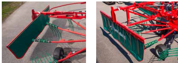
Automatic fold-able swath board with parking stand.
