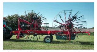
With its' clever folding mechanism the total height remains below 4.00m - despite a rotor diameter of 3.85m. And there is no need to remove tine arms for road transport.
