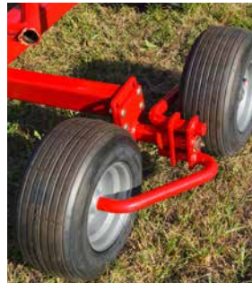
Optional boogie wheels for the Quattro undercarriage for further improved ground contour following.
