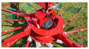
Each rotor can be independently and hydraulically set for height. A minimum height can be mechanically adjusted as well to secure correct setting.
