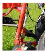
Standard oscillation dampers ensure excellent running characteristics.
