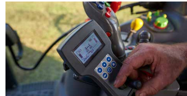
ComfortKit including electronic control of individual rotor height.
