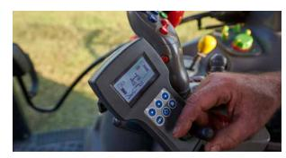
ComfortKit including electronic control of individual rotor height.
