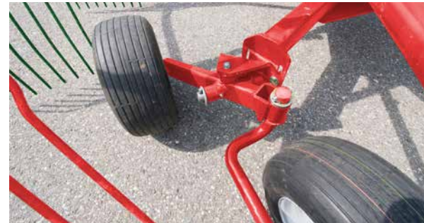
Optional tandem axle for additional stability especially on hillsides.
