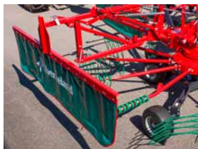
Automatic fold-able swath board with parking stand.
