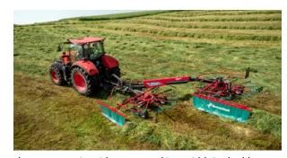
The 9671 S Vario with 7.10m working width in double swath position.
