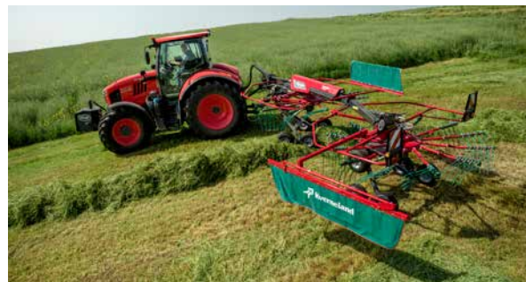
Turning on headlands: Kverneland is equipped with the QuickLift system as standard. This ensures a lifting height of 50cm to easily over cross existing swaths.
