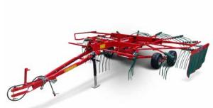
Kverneland 9447 T with 4.70m working width and a weight of only 665kg.
