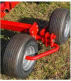
Optional boogie wheels for the Quattro undercarriage for further improved ground contour following.
