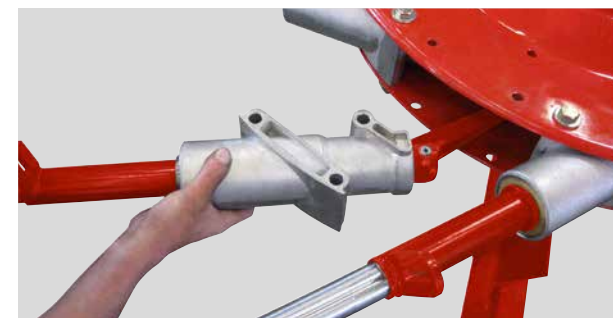
Each ProLine tine arm can be dismantled and repaired individually.
