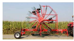
With 9.00m working width and transport height below 4.00m, even without detaching tine arms...
