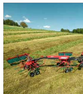
SideShift to the left - raking without driving on the crop.
