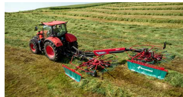
The 9671 S Vario with 7.10m working width in double swath position.
