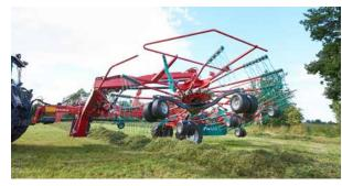
High lift of rotors ensures generous clearance during headland turns. Clearance height can be adjusted.
