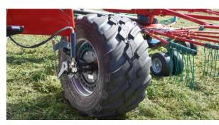
The optional active wheel steering provides excellent manoeuvrability during narrow gateways and tight corners.
