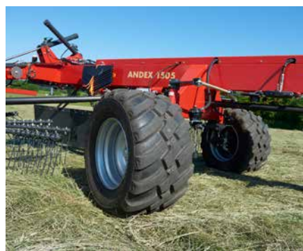
The optional active wheel steering provides excellent manoeuvrability during narrow gateways and tight corners.
