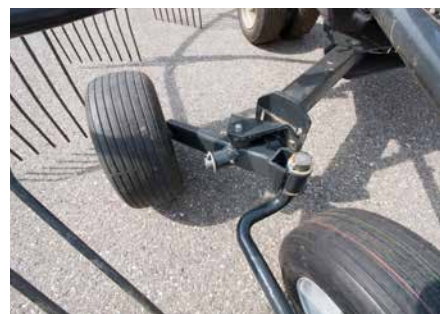
Optional tandem axle for additional stability especially on hillsides.
