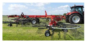
Each rotor can be independently and hydraulically set for height. A minimum height can be mechanically adjusted as well to secure correct setting.
