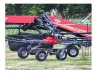
The Touch-Down-Effect, comparable to an aircraft's approach angle of its landing gear, ensures smooth and clean raking, but with lifting to a ground clearance of around 500mm avoids that swaths on headlands are damaged.
