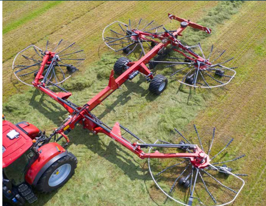
The unique elbow construction positions the front rotors close to the driver for excellent overview.
