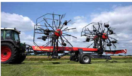
Vicon Analex 1254 Hydraulic lowerable for transport below 4m.
