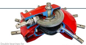
crown wheel and Maintenance-free cam track and tine arms, running in an oil bath.
