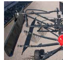
Automatic fold-able swath board with parking stand.
