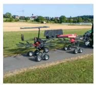
Pulled axles ensure smooth handling and low frame stress on both road and field.
