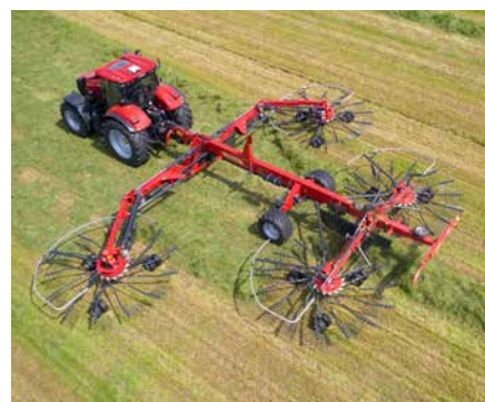
The two outer rotors can be adjusted individually to obtain working widths between 9.8-15.0m.
