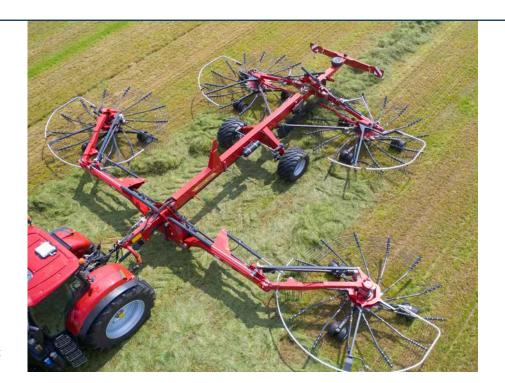
The unique elbow construction positions the front rotors close to the driver for excellent overview.
