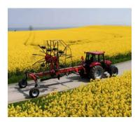
Vicon centre swath rakes are converted hydraulically for transport from the tractor cab.
