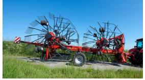
**Vicon Andex 1505 Plus**Clever folding mechanism for road transport.
