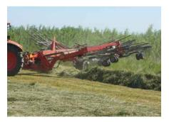
High lift of rotors ensures generous clearance during headland turns. Clearance height can be adjusted.
