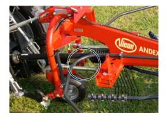
Oscillation dampers ensure excellent running characteristics.
