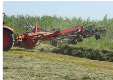
High lift of rotors ensures generous clearance during headland turns. Clearance height can be adjusted.
