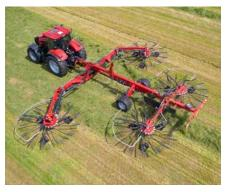
The two outer rotors can be adjusted individually to obtain working widths between 9.8-15.0m.
