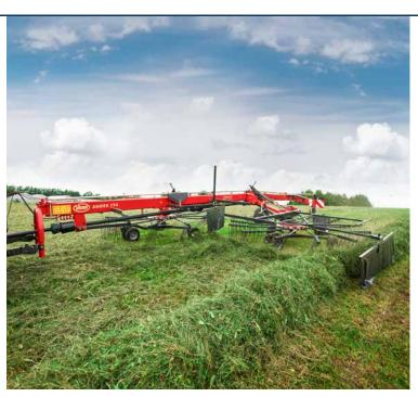
The side delivery concept allows you to collect crop from 15.00m into a single swath.
