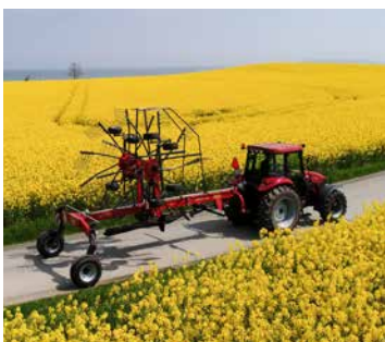
Vicon centre swath rakes are converted hydraulically for transport from the tractor cab.
