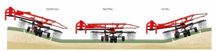
The rotors are fully flexible in all directions, which means the tines have exceptional ground following ability....
