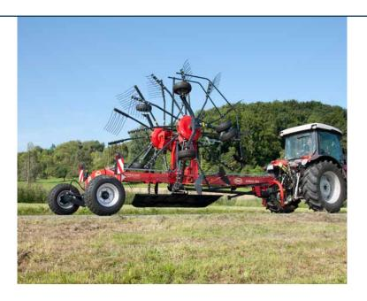
Add in features such as adjustable working width of 6.2-7.2m, TerraLink Quattro ground contour following and heavy duty carrier frame design, and the result is low maintenance, higher productivity and maximum operator comfort.
