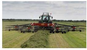
Working width can be set hydraulically between 10-12.5m. Swath width is also set hydraulically between 1.2 and 2.2m.
