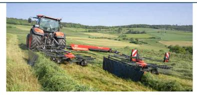
The 715T Vario with 7.10m working width in double swath position.
