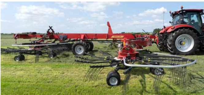
Each rotor can be independently and hydraulically set for height. A minimum height can be mechanically adjusted as well to secure correct setting.
