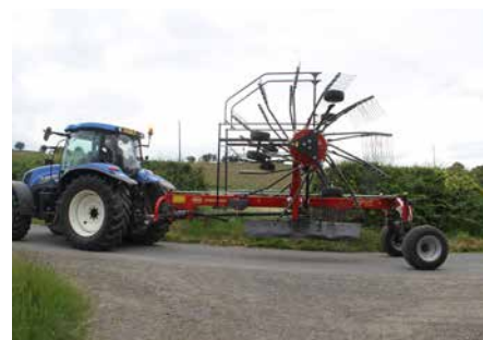
The AnDEX 804 includes a transport height below 4.00m without leaving the tractor cab. Actively steered axles support tight turns on headlands and during transport.
