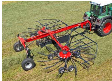
Andex 844 with 8.40m working width, fully enclosed gearbox and hydraulically adjustable working width.
