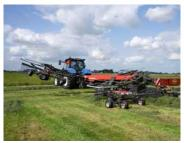
With the individual lifting feature of all four rotors awkward shaped fields can be raked efficiently and cleanly.
