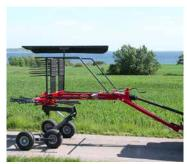
With a linkage mounted drawbar, the Andex 474T and 424T can be easily operated by low horse power tractors.
