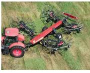
The high lift of the rotors ensures generous clearance during headland turns and allows sharp turns up to 80°
