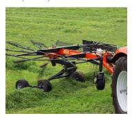
The machine can conveniently be raised up to a height of 50cm from the tractor driver's seat.
