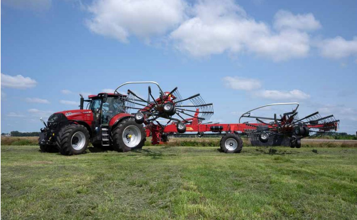
All four rotors can be lifted individually.
