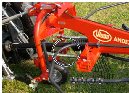
Oscillation dampers ensure excellent running characteristics.
