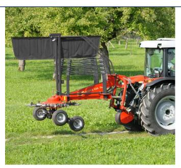
For transport or storage, the rotor guard frames are folded up close to the mainframe, locking automatically into position. An assistor spring linked to the swath board reduces the effort required.
