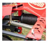
A pivoting 3-pt headstock ensures perfect ground following performance, and perfect tracking when cornering. Oscillation dampers are optionally available.
