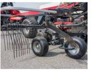
With electric rotor height adjustment the min and max height is indicated as a percentage. It is possible to set your own zero point, to avoid accidentally raking lower than your field conditions allow. Lowering beyond this point will be shown on screen as a negative percentage.
