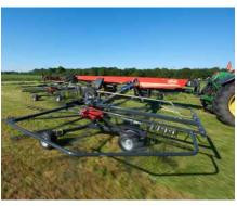
TerraLink Quattro is a unique combination of flexible frame arm and 3-dimensional rotor suspension
