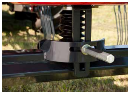
Infinitely variable cam track adjustment allows fine tuning, to obtain optimal raking and swath formation according to crop conditions.
