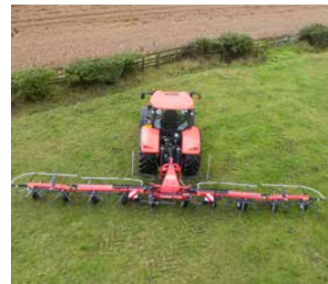
New folding mechanism – ensures even weight distribution during the complete folding sequence.
