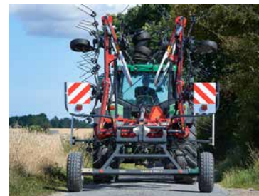
Standard running wheels of Fanex 904C are extra wide 10.0/75 – 15.3 tyres with a generous track width of 2.45m.
