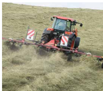
With the optional reduction gearbox it is possible to place night swaths.
