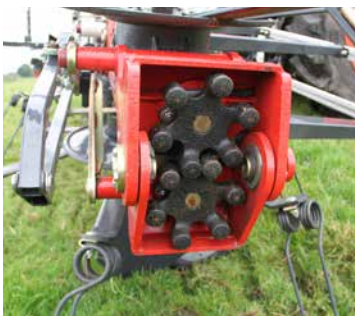
Fanex 1124 is fitted with the XL version of HexaLink finger clutch.
