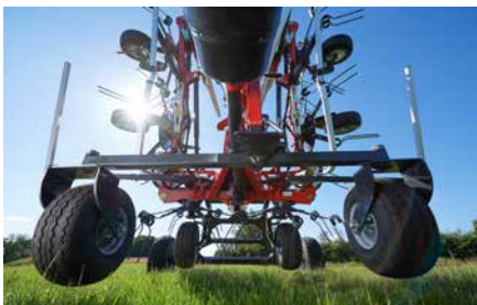
New optional third wheel with tandem axle for high accuracy in ground followings.
