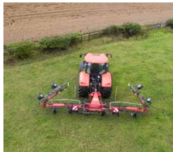
New folding mechanism – ensures even weight distribution during the complete folding sequence.
