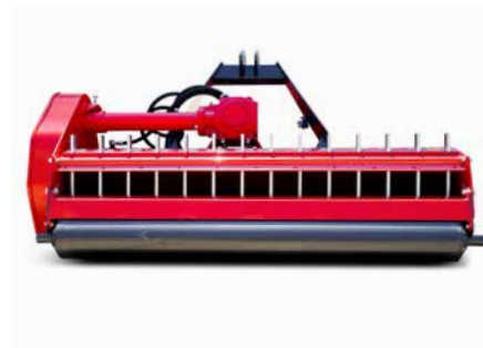
The Vicon Bromex PM can be equipped with rake tines to improve chopping on prunings.
