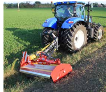
Tilting angle of -65 degrees.
