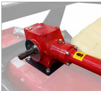
All gearboxes on Vicon choppers range feature as standard an integrated free wheel.
