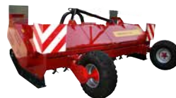
Agri Choppers (Bromex CZ) 3.20-4.00m working width
