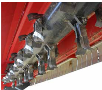
Special hammer design or fan or universal blades create a suction effect lifting material and improving cutting.
