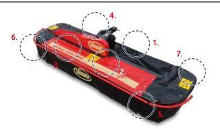
to stable and smooth running of the tractor, when going up and down steep slopes. The suspension concept allows a transverse adaptation of 28°. giving the mower outstanding flexibility.
