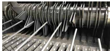
15% Bigger intake rotor with 15 knife SuperCut pre-chopping system.
