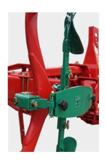
The new generation of Kverneland ploughs feature legs with a new design, called "aero-profile". Not only higher than the standard Kverneland legs, these new legs improve the soil flow. Heavy residues are pushed out, hence limiting possible blokages even with 85 cm interbody clearance.
