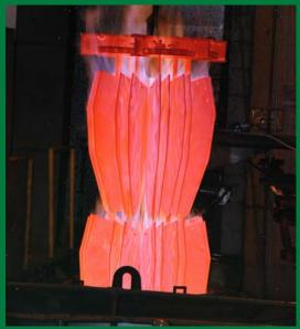
Kverneland 12 hours carburising process results in creating 2 steels in 1 sole mouldboard.
