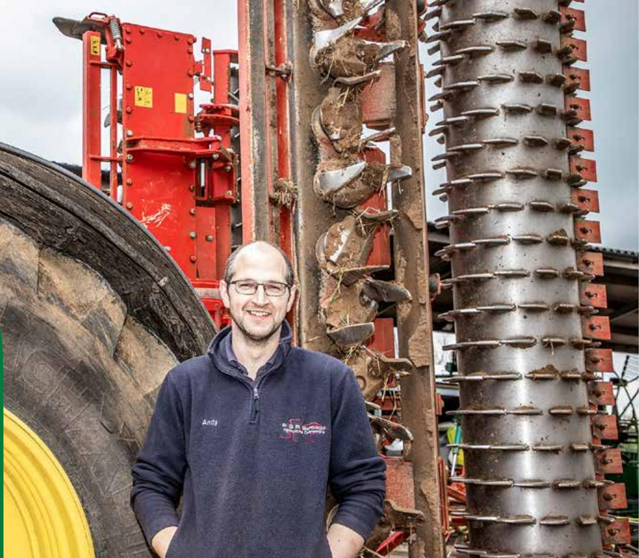
Foreman Andy Russell says the power harrow doesn't leave ridges thanks to heavy duty spring-loaded side-deflectors, and the toothed packer roller provides a good firm finish in almost any soil type encountered.
