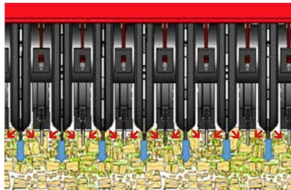
The ring and shoulder angle design of the Actipack roller provides consolidation to depth without tightening up surface aggregates. Provides good weathering effect and transition of moisture through profile.
