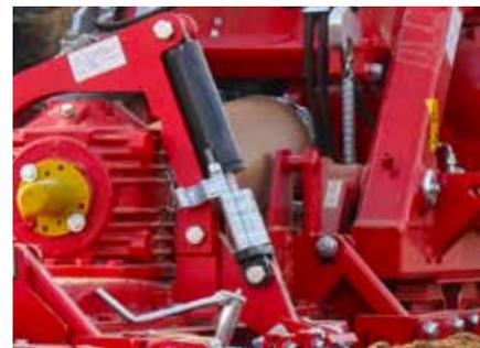
On the hydraulic foldable power harrows the working depth setting is adjusted by spacers at the cylinders. The working depth is changed hydraulically from cab. A parallelogram linkage ensures that the power harrow is always in a horizontal position to the roller. Therefore, the packer roller scraper bar position is basically a fixed height to the ground, independent from the working depth.
