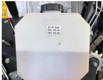
Large capacity chain lube tank.
