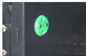
Moisture sensors located inside bale chamber.
