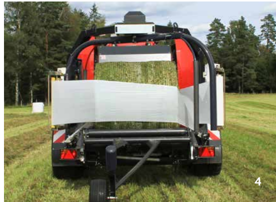
The wrapping table moves very fast to the pre-stretchers and wrapping starts instantly.
