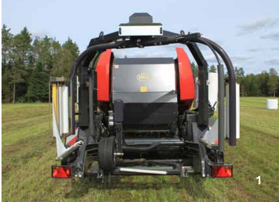
Once the net is applied to the bale the wrapping table is transferred to the tailgate of the baler.
