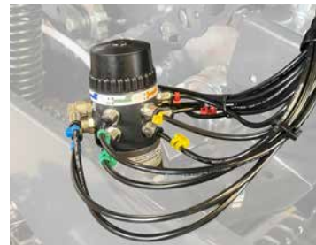
Automatic chain lubrication with individually adjustable outlets.
