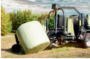
Bale turner option. During transport the kit is automatically pivoted into a safe position on the wrapping unit.
