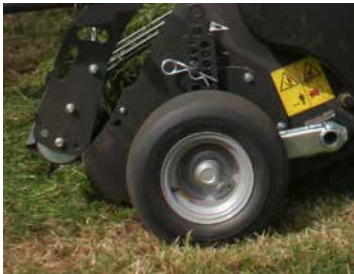
Generous flotation tyres with simple height adjustment.
