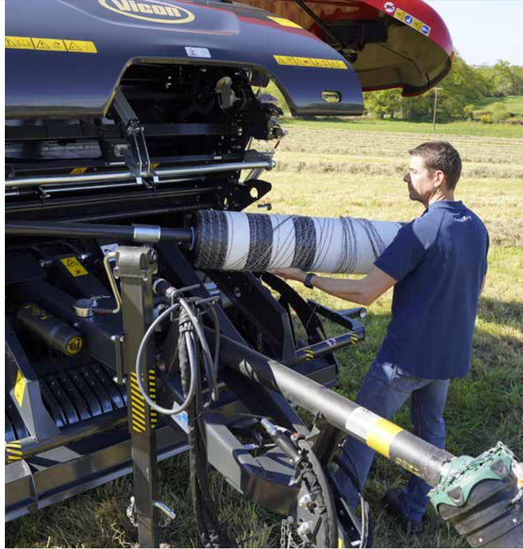
Very low loading height and easy threading of the system make for minimum downtime and maximum time baling.
