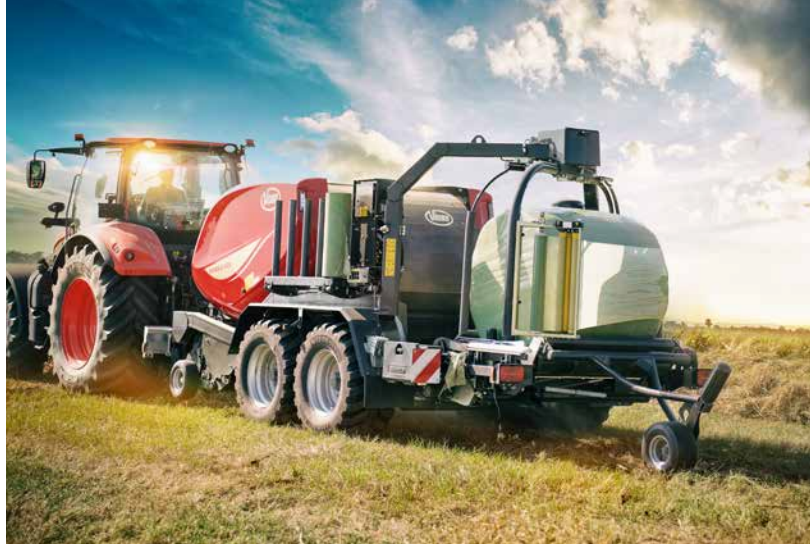
Twin satellite wrapper with 2 pre-stretchers and 4 endless belts for fast and stable wrapping.
