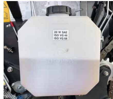
Large capacity chain lube tank.
