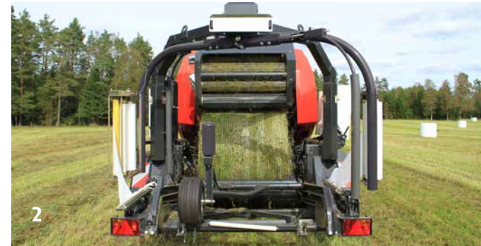
The bale is dropped directly onto the wrapping table.
