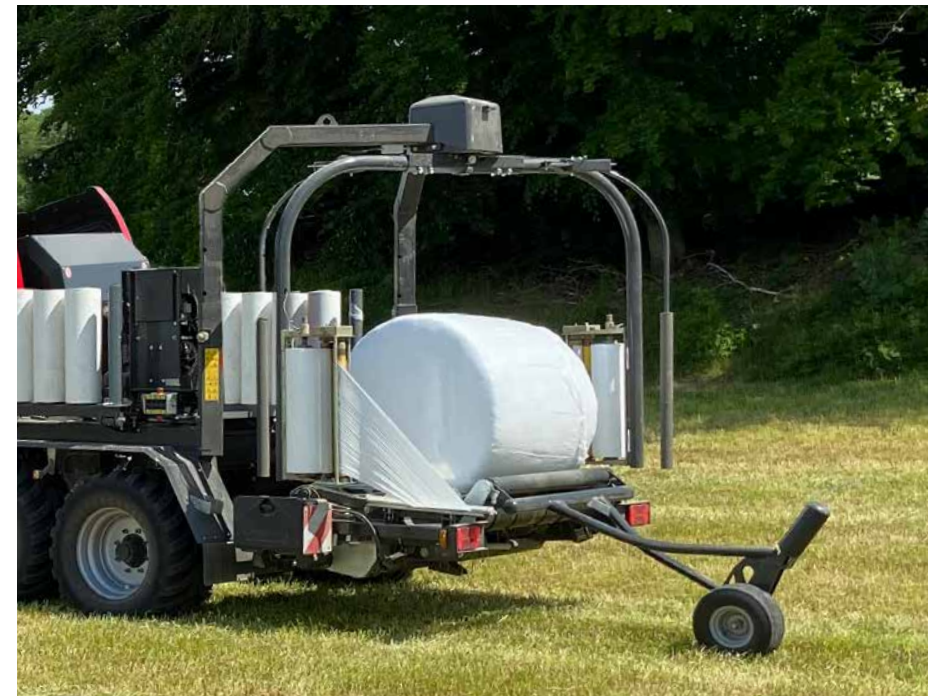
Twin satellite wrapper with 2 pre-stretchers and 4 endless belts for fast and stable wrapping.
