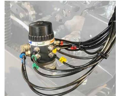
Automatic chain lubrication with individually adjustable outlets.
