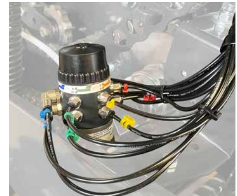
Automatic chain lubrication with individually adjustable outlets.
