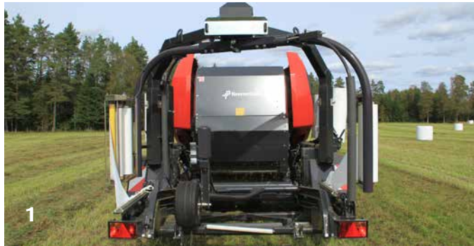
Once the net is applied to the bale the wrapping table moves forward under the tailgate of the baler.
