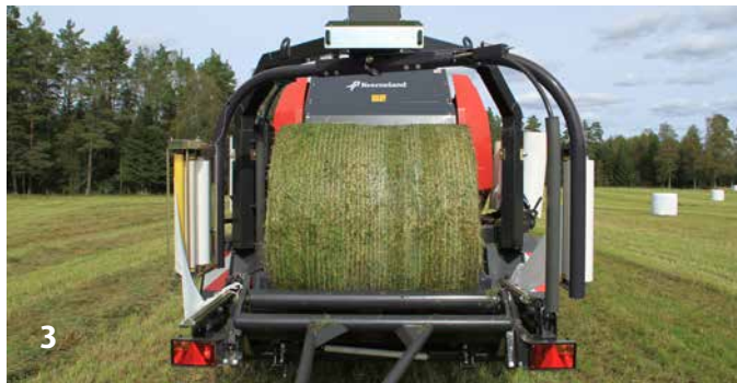
As soon as the bale is transferred away from the baler, the tailgate automatically closes, and baling can resume.
