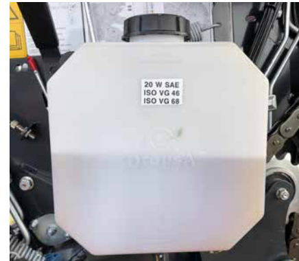
Large capacity chain lube tank.
