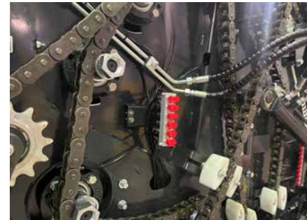
Remote grease bank for bale chamber roller bearings.
