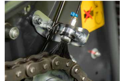
Automatic chain lubrication is standard on Kverneland 6500F.
