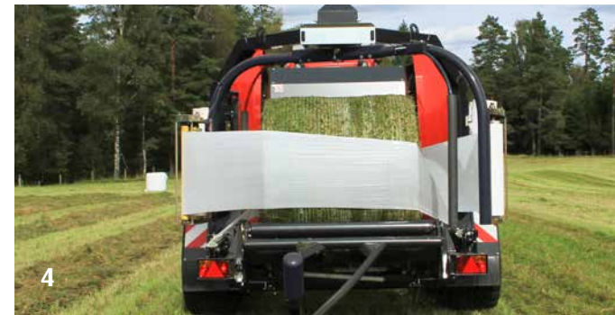
The wrapping table moves rapidly to the pre-stretchers and wrapping starts instantly.
