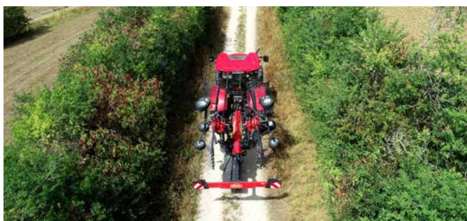
Position de transport compacte.
