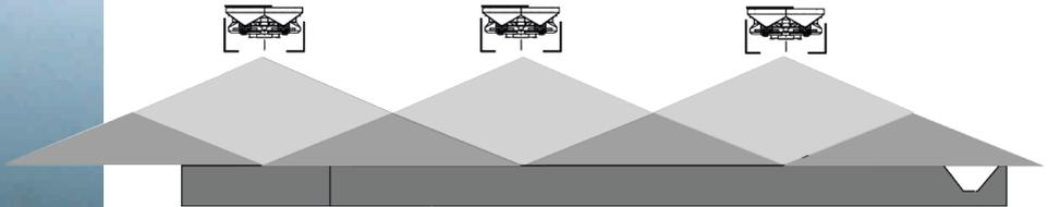
*Triangular shaped spreading pattern: complete overlap between passes*
