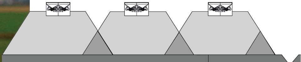
*Trapezium shaped spreading pattern: partly overlap between passes*
