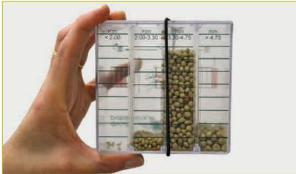
*Granular size box to measure the fertiliser distribution*
