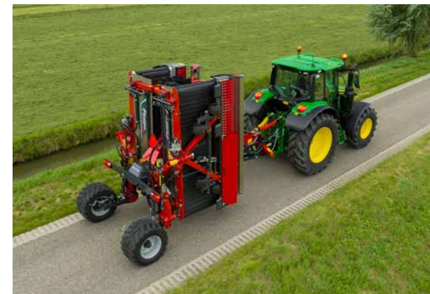
The Kverneland Roc 1073 S can be folded into a width of only 2.5 meters for road transport.
