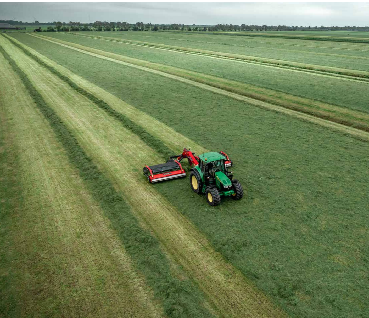
The Kverneland Roc 1073 S can be folded into a width of only 2.5 meters for road transport.
