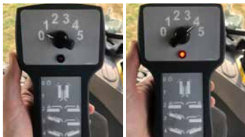
All hydraulic functions are controlled via the tractor valves in combination with a pre-selection PilotBox.
