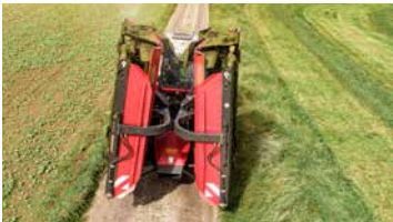
The machine folds into a an above 90° transport position, keeping the mowing units away from treetops.
