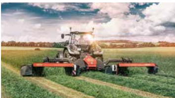
Vicon EXTRA 787T QuattroLink triple mower combination with 8.75m working width.
