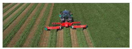
Kverneland 5387 MT QuattroLink triple mower combination with 8.75m working width.
