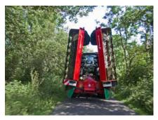
The machine folds into a an above 90° transport position, keeping the mowing units away from treetops.
