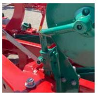
The adjustment is done by loosening the bolt on the clamp followed by adjusting the disc up or down.
