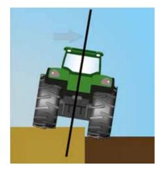
**Different tyre pressure**Gives a different angle when ploughing left and right.
