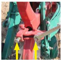
Adjusting the tie rod is done by the two bolts shown above.
