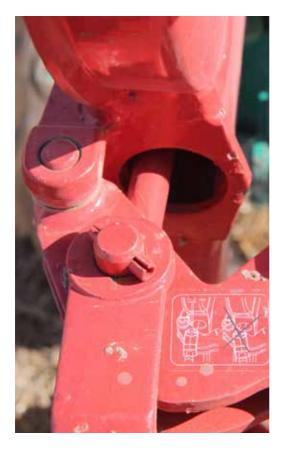
The distance between the tie rod and the anchor should be 1-2 mm.
