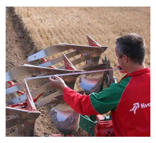
Check the furrow width by measuring the distance between the landside and the point.
