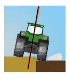
**Identical tyre pressure**Gives the same angle when ploughing left and right, for the best ploughing results.
