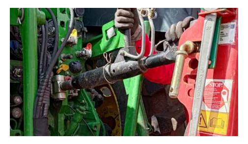
The length of the top link must be adjusted so that the plough is parallel to the ground.
