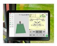
The Isomatch Tellus 700 is for forage machines the most recommended due to the blister buttons in addition to the touch screen. Operation without watching the screen is due to the real buttons possible. Also, our terminal can be used with other ISOBUS implements, like for example, sprayers and spreaders. Not only out of our product range, as well from competition, as long they comply to the ISOBUS standard.
