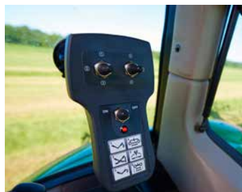
Single side lift front rotors incl. hydraulic suspension of front rotors
