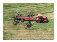
Compact but efficient machine – in combination with BX mower there is possibility to collect up to 20m into one swath.
