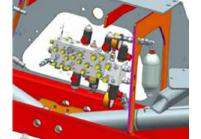
Single side lift front rotors incl. hydraulic suspension of front rotors
