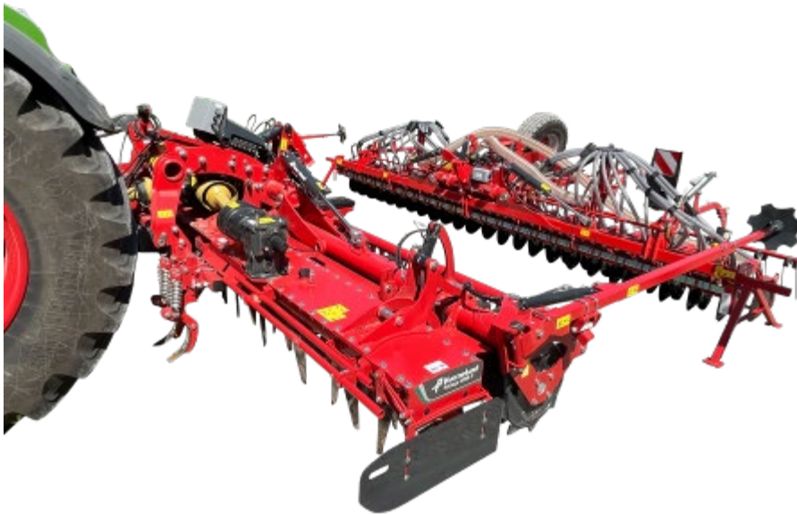
Kverneland coulters bar f-drill CB F with easy CAT. II connection
