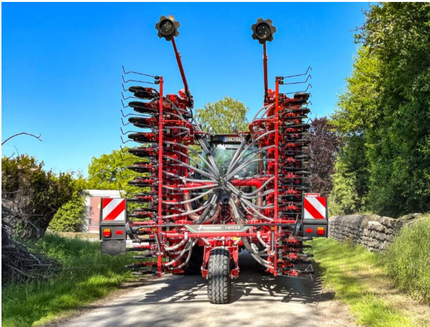
Kverneland coulters bar f-drill CB F safe road transport with support wheel
