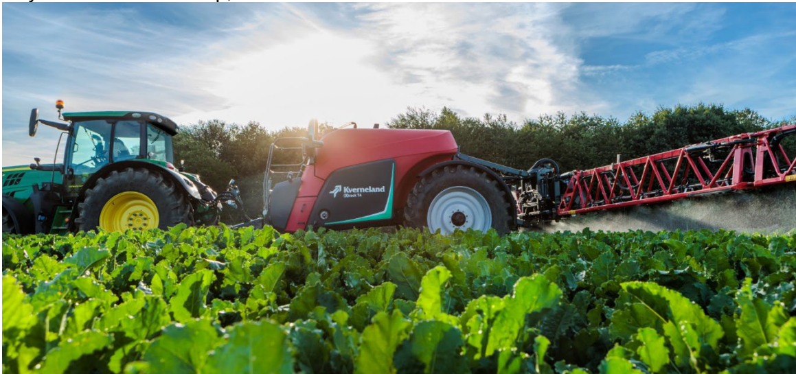
iXtrack T4 with the new nominal tank capacity of 5300 litres, improving efficiency and performance
