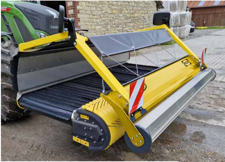
Working width 3.8m (12'6") and transport width 2.95m (9'8").
