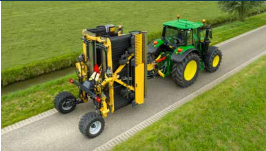
The Vicon ROC RS 730 can be folded into a width of only 2.5 meters for road transport.
