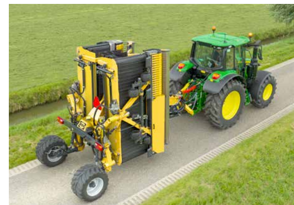
The Kverneland ROC RS 730 can be folded into a width of only 2.5 meters for road transport.
