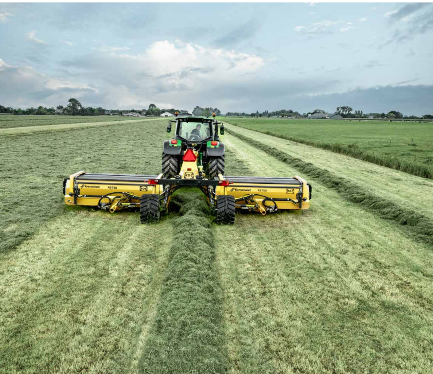
The Kverneland ROC RS 730 can be folded into a width of only 2.5 meters for road transport.
