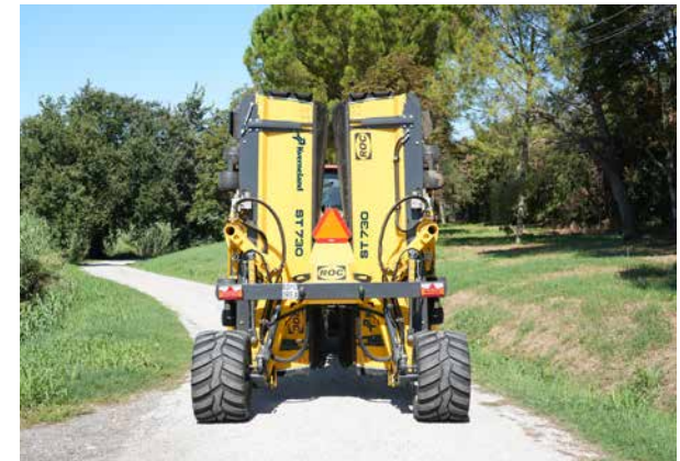
The Kverneland ROC ST 730 can be folded to a width of only 2.5 meters for road transport.
