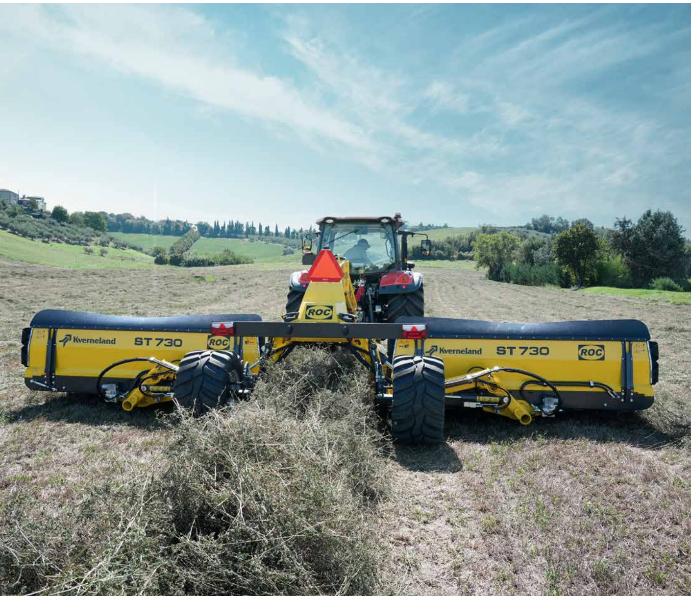
The Kverneland ROC ST 730 can be folded to a width of only 2.5 meters for road transport.
