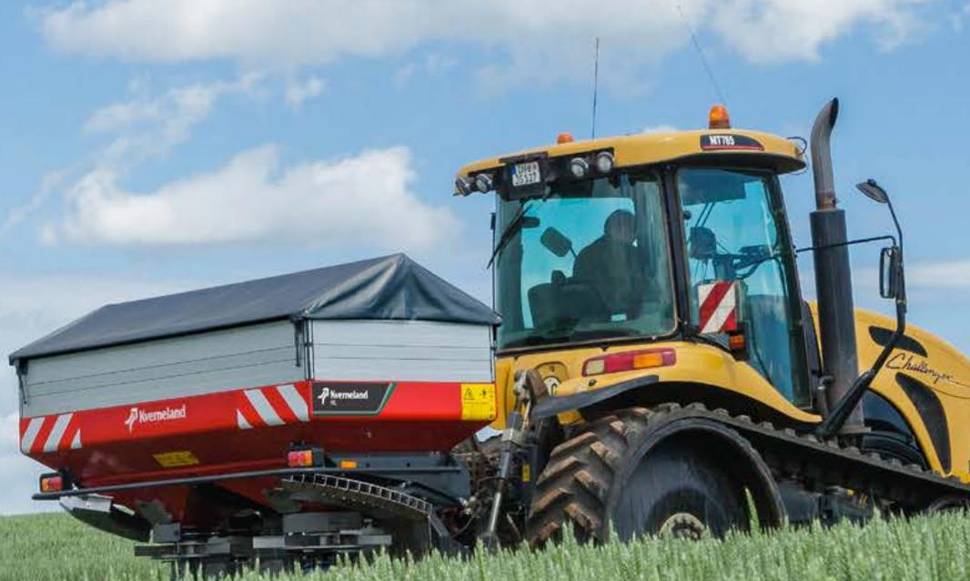
The Remote Control II spreading computer provides all the functions to start and stop the spreader, to set the right application rate and to increase and decrease the application rate on the move. The latest settings are retained in the memory function. Both discs can be shut off independently to spread half the working width.
