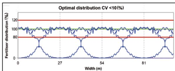
A CV <10% means an optimal spreading pattern
