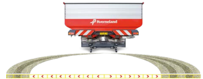
Switching off the sections outwards
