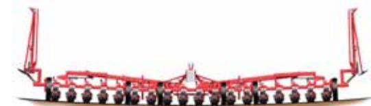
18-rows parallel-hydraulic folding frame; 9.0m working width.
