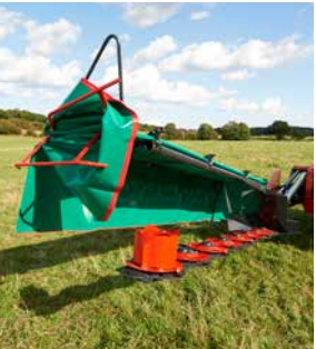
Easy access to the cutterbar for inspection and maintenance.
