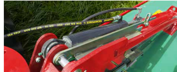
Headland lift via hydraulic cylinder.
