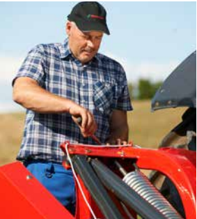
Ground pressure is easily set by adjusting the compensating spring.
