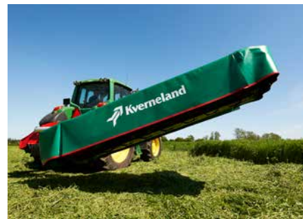
Lifting on headlands via hydraulic cylinder – ample ground clearance.
