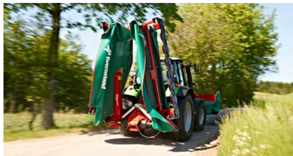
Vertical transport position for good weight distribution.
