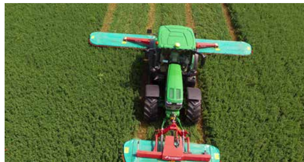
Centre suspended design for excellent ground following ability.
