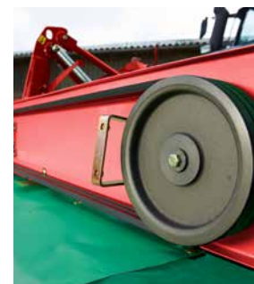
By switching pulleys changing between 1000 and 750rpm is possible.
