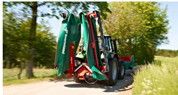
Vertical transport position for good weight distribution.
