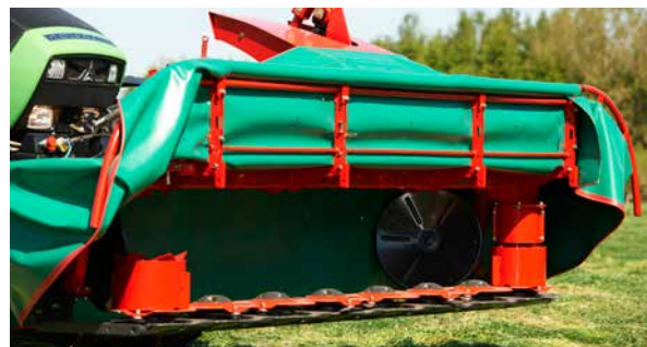
Easy access to the cutterbar with foldable front and side guards.
