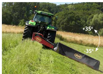
The design allows mowing at extreme angles.
