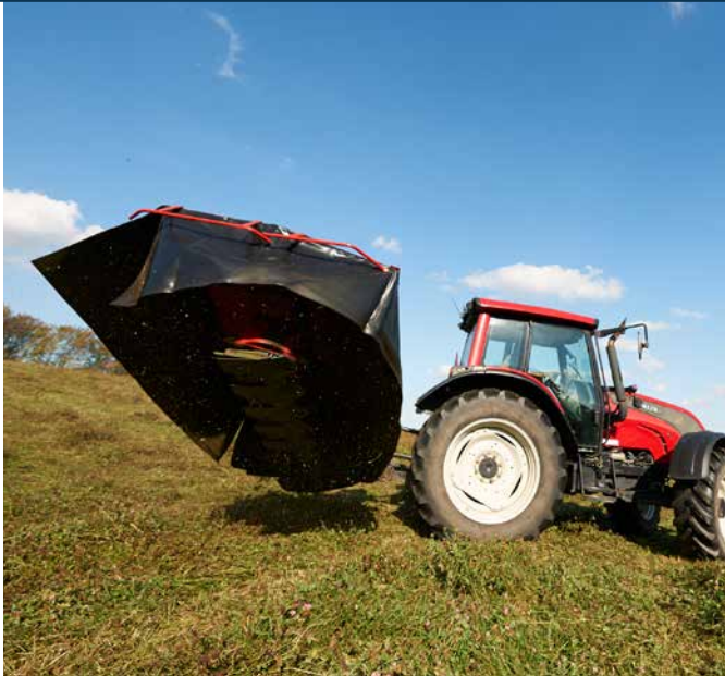
Lifting on headlands via a hydraulic cylinder.
