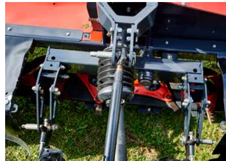
Pivoting point positioned in the axis of center of gravity for excellent ground tracking and even ground pressure across the complete width.
