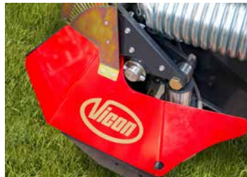
Hydraulic on-the-go setting of ground pressure (optional).
