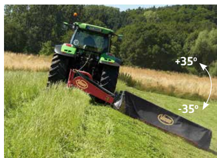
The design allows mowing at extreme angles.
