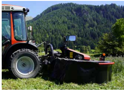
Gravity point is close to tractor for stable, safe operation on steep slopes.
