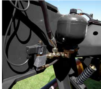
Hydraulic suspension ensures precise setting of ground pressure (EXTRA 440H).
