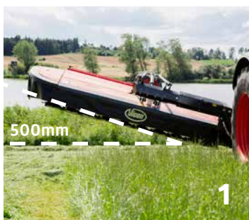
Minimum 500mm ground clearance across the complete mowing unit during headland turns. Mowing unit is raised and carrying arm tilted to a 10° angle.
