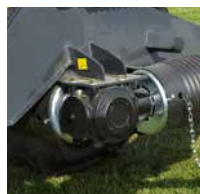
540/1000rpm turnable gearbox as standard.
