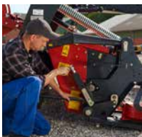
Easy adjustment of stubble height.
