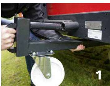
Slide the purpose-built transport rollers onto the BX-belt and remove the connection pin.
