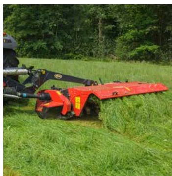
Quick change from swathing to widespreading.
