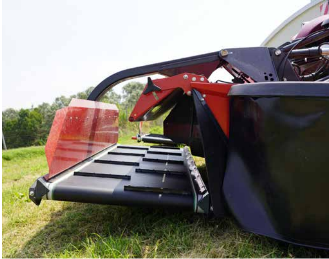
The wide belts allow handling of heavy crop flow.
