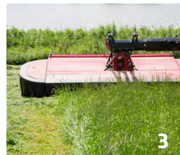
Mowing unit is lowered evenly onto the ground without one side touching the ground before the rest of the mower.
