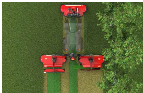
Using one belt to move crop away from field boundaries.
