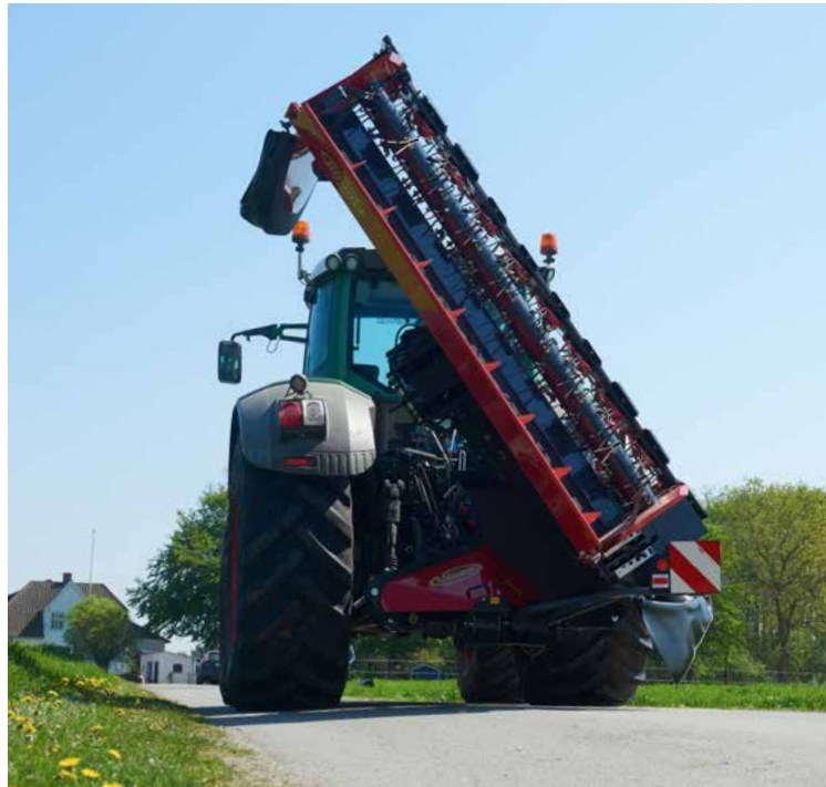
EXTRA 736T Vario in transport. The telescopic frame arm moves to the lowest possible position to reach a transport height of only 3.70m
