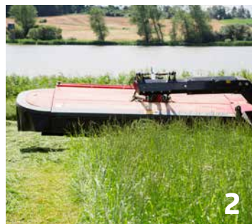
The carrying arm is tilted back to bring the mowing unit into an even position before lowering the mowing unit.
