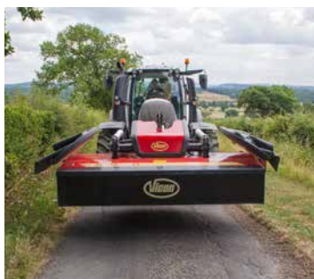
Hydraulic folding of FlexProtect guards (optional).
