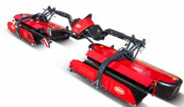
Triple Mower Conditioners 10.20m working width
