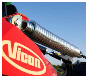
The large compensating spring ensures excellent flotation across the full mower width.
