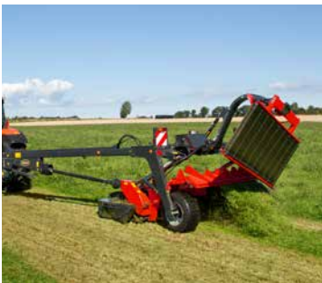
When placing the first swath, the belt is raised and hydraulically lowered for the second swath.
