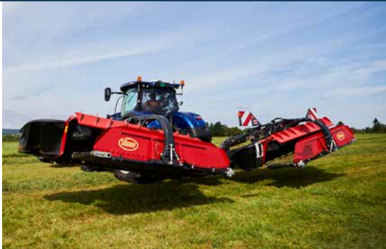
AutoStop function of the BX belt is activated when raised on headland to reduce fuel consumption.
