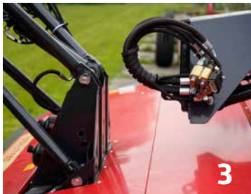
3 Lower the mowing units and the BX belt automatically comes off.
