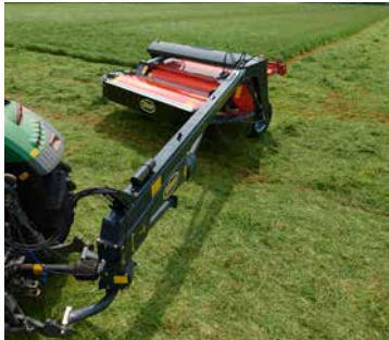
The swivel hitch headstock with reversible gearbox provides optimal manoeuvring ability.
