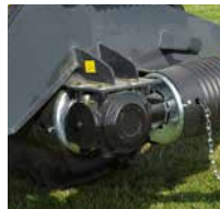
540/1000rpm turnable gearbox as standard.
