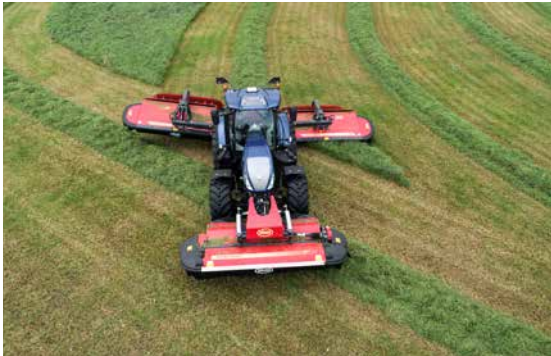
When using one belt only, speed is reduced to avoid crop being placed too far across the middle.
