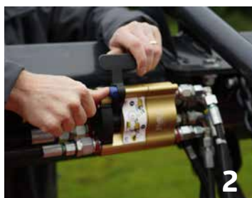
Disconnect the power cable and all hydraulic connections to BX belt with one single lever.
