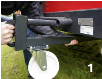
1 Slide the purpose-built transport rollers onto the BX-belt and remove the connection pin.
