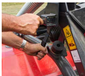
One-touch parking handle, to lock and prepare the machine for dismounting.
