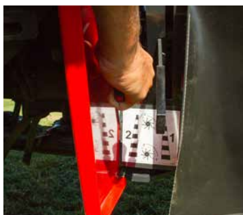
Dual adjustment of conditioner plate to customize to crop intensity.
