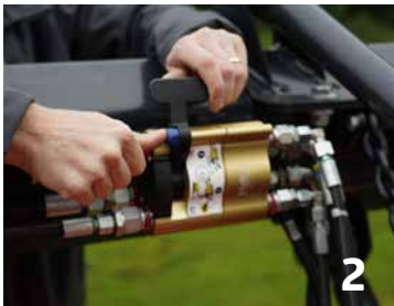
2 Disconnect the power cable and all hydraulic connections to BX belt with one single lever.
