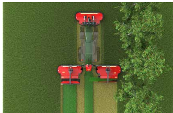
Using one belt to move crop away from field boundaries.
