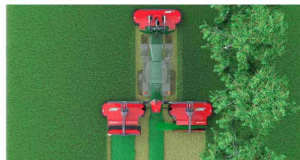
Using one belt to move crop away from field boundaries.
