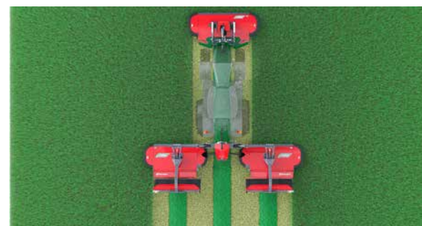
Three single swaths, easy set with the integrated swath plates.
