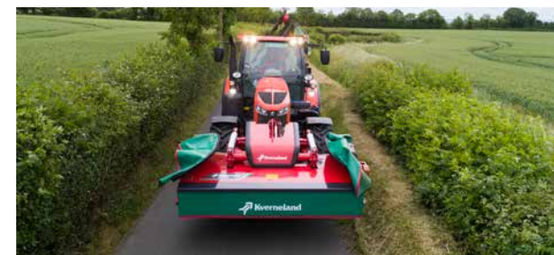
Hydraulic folding of FlexProtect guards (optional).
