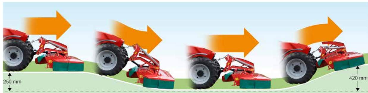
Excellent down- and upwards ground following ability of 250mm and 420mm respectively.
