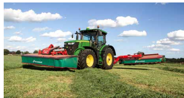
AutoStop function of the BX belt is activated when raised on headland to reduce fuel consumption.
