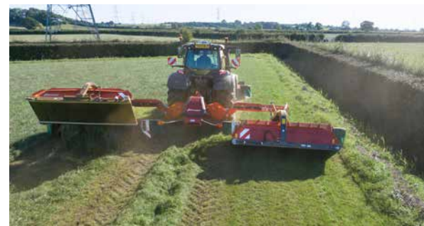
When using one belt only, speed is reduced to avoid crop being placed too far across the middle.
