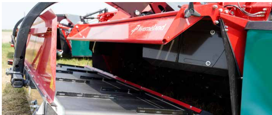
The wide belts allow handling of heavy crop flow.
