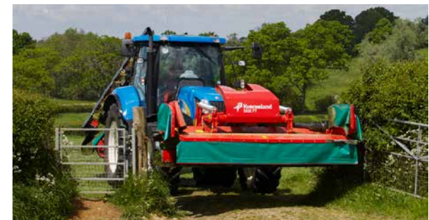
Foldable sideguards ensure narrow transport width.
