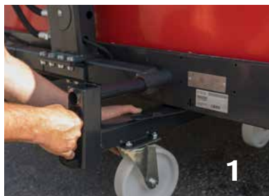
Slide the purpose-built transport rollers onto the BX-belt and remove the connection pin.
