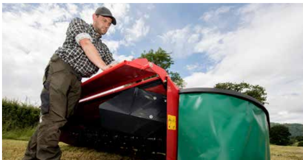
Integrated swath plates, easily adjusted to correct swath width.
