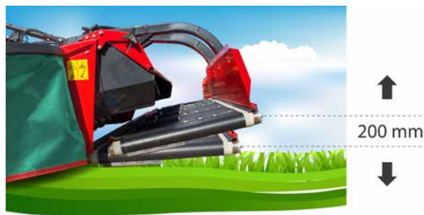
Vicon BX can deliver the crop at different working height.
