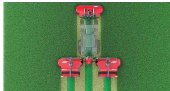
Three single swaths, easy set with the integrated swath plates.
