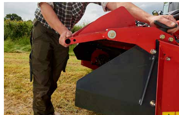
Swath plates automatically expand when being slid inwards to support efficient and accurate swathing.
