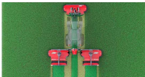
100% wide spreading with the standard fitted FlipOver spreading vanes.
